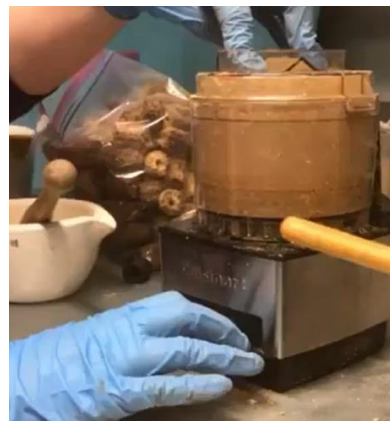
Figure 2-5: Grinding corn larger than the 250- \mu\text{m} sieve with a mini food processor
