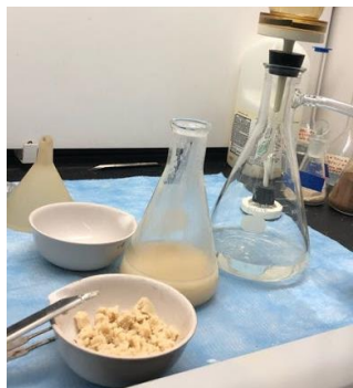
Figure 2-10: Dried NaOH saturated nitric acid treated corn cob with filtration
